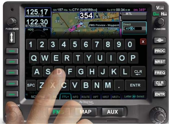
A pop-up QWERTY-style keyboard automatically appears when an alpha-numeric data field is highlighted, making data entry as familiar to you as your computer or smart phone. With GeoFill, the IFD540 will virtually always guess accurately your next waypoint after only entering one or two letters.
