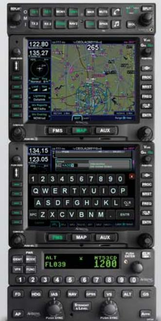
*Built on a dual databus architecture, the IFD540s are key components in Avidyne's new panel-mounted avionics suite, which also includes the AMX240 Audio Panel and AXP340 ADS-B Extended Squitter Mode S Transponder.*
