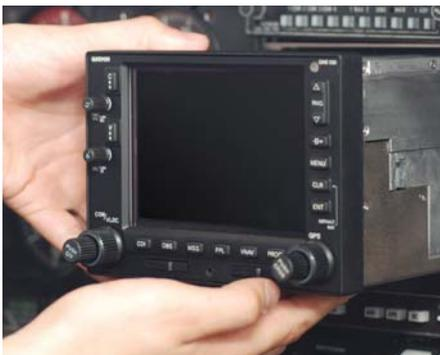
The IFD540 is designed as a plug & play replacement for the popular GNS530 & 530W navigators, but with bigger glass, a much larger screen area, 400% more pixels, and a much easier to use hybrid touch screen interface. And because it's the same physical size, uses the same tray & antennas, and can be installed with no wiring changes, it makes it an incredibly easy and affordable retrofit for general aviation aircraft.
