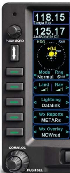
Versatile dual-sided Line Select Keys provide easy control of the thumbnail Hazard Display and map overlay settings. Dual-concentric knobs, dedicated function buttons, and a highly-intuitive touch-sensitive display combine to give pilots a datalink-enabled, map-centric view of their flight situation, while providing quick access to all of the IFD540's powerful functions.
