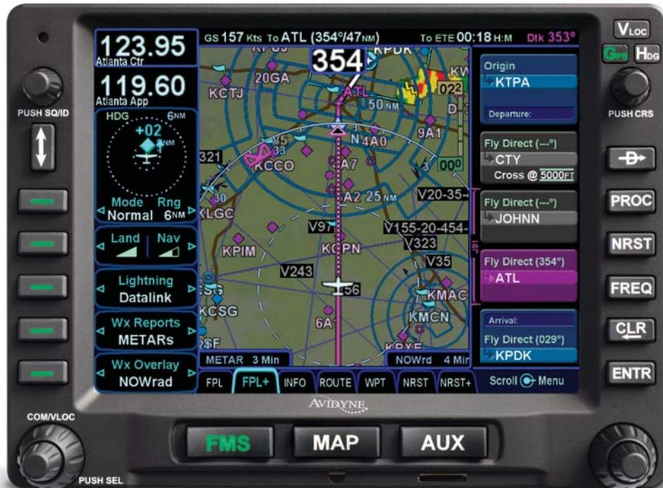
*Avidyne's IFD540 FMS/GPS/NAV/COM combines the best Flight Management System available, with a multi-channel digital VHF radio, in an easy-to-use, plug & play design.*
