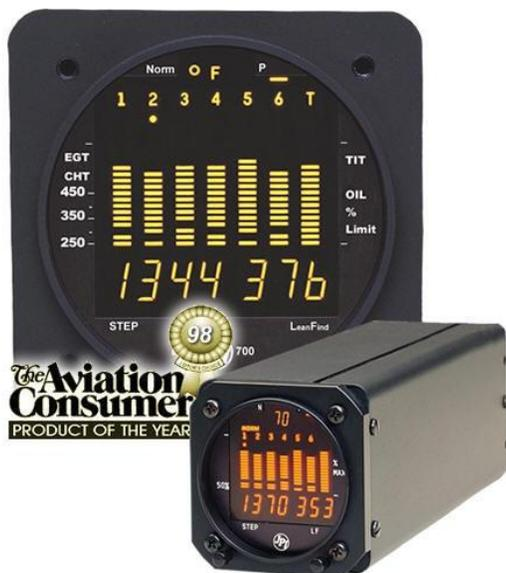
The Engine Data Management 800 system is the most advanced and accurate piston engine-monitoring instrument on the market. Using the latest microprocessor technology, the EDM will monitor up to twenty-four critical parameters in your engine, four times a second, with a linearized thermocouple accuracy of better than 0.1 percent or 2 °F.
