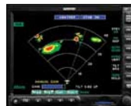
Weather data from the GWX 68 digital radar is displayed on compatible Garmin MFDs via ARINC 429/453 interface.
